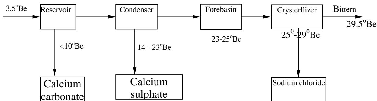
${}^{\circ}\text{Be}$ -Reading of Baueme hydrometer
